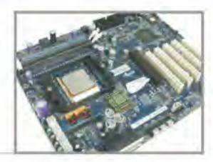
Remove the two screws from the retention module.
